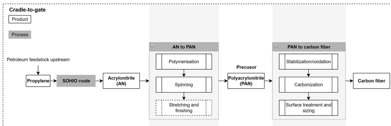
Fig. 2. Typical manufacturing processes for PAN-based carbon fiber (adapted from [Dér et al., 2021](#); [Huang, 2009](#); [Morgan, 2005](#)). Manufacturing carbon fiber from other precursors, such as pitch and lignin, involves different processes. In the figure, processes shown with solid lines indicate the availability of energy demand data, while those with dashed lines indicate the absence of such data. Both will be further elaborated in [Section 3.2](#).
