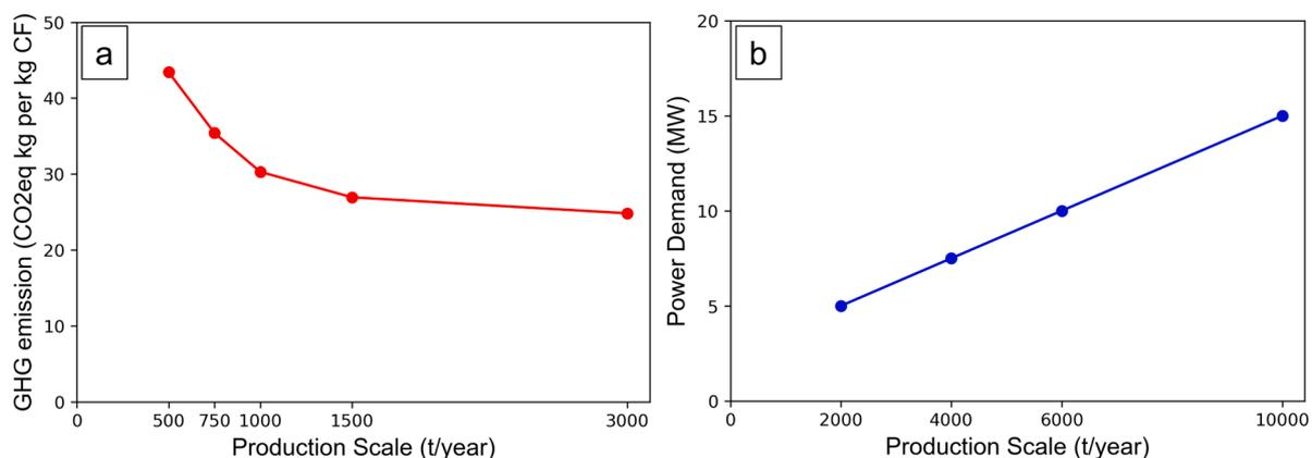
Fig. 3. Relationship between carbon fiber manufacturing production scale and (a) greenhouse gas (GHG) emissions (CO<sub>2</sub>-eq per kg of carbon fiber) and (b) power demand (MW).
